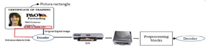
Fig.1. Overall schematic of the proposed ID card based authentication system.
